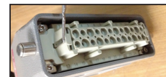
Photos 2 & 3 – Ground Location on Connectors
