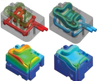
TruCool conformal cooling provides superior heat transfer over conventional cooling technologies.
