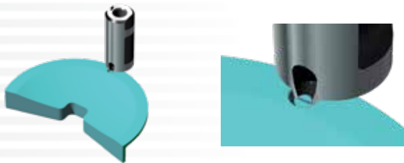
Flat Part with Companion Vestige – installation in fixed half of the mold
