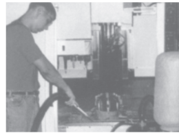
The Chip Vac removes abrasive stainless steel chips from a CNC.
