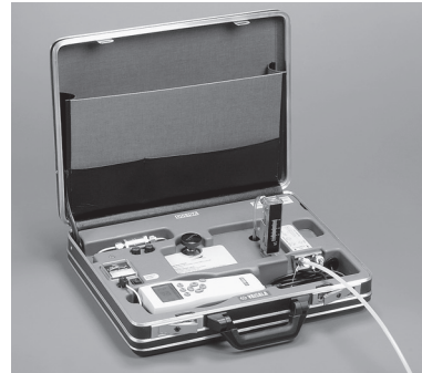
The DSS70A provides a compact solution for field checking dewpoint where direct measurement is difficult.
