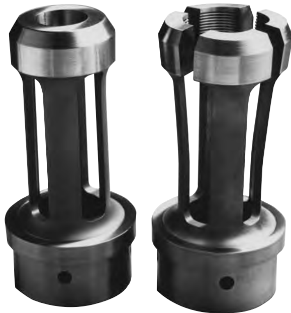
The Expandable Cavity is maintained under compression during molding.
