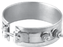
TYPE W3-B Post Terminals Both posts on one side of gap Minimum I.D. - 1 1/2" Minimum width - 3/4"
